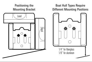
NOTE: If you have a flat-bottomed aluminum boat, some additional adjustment may be needed to accommodate the rivets on the bottom of the boat (i.e. the gap may need to be a little smaller than 1/8"). This will help you to avoid excessive turbulence at high speeds.
